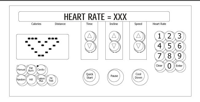
Upon initial entry to this test, a message concerning the telemetry system on/off will occur. This test will allow the user to test the telemetry heart rate system. If the telemetry heart rate system is OFF, no heart rate value will be given.
